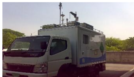
Mobile Air Quality Monitoring Station
